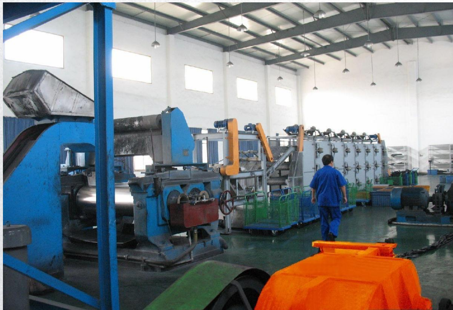
Rubber mixing semi-automatic production line
